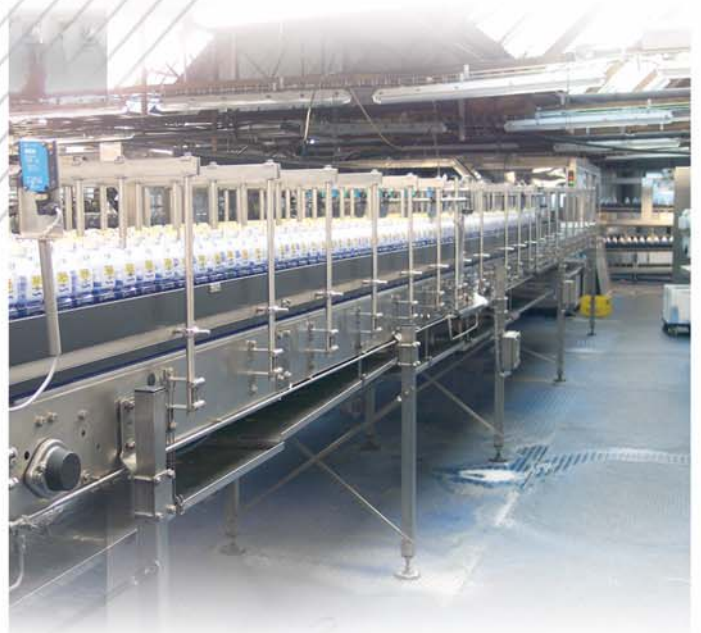
LINEAR TRANSFER WITH FLOWFLEX
